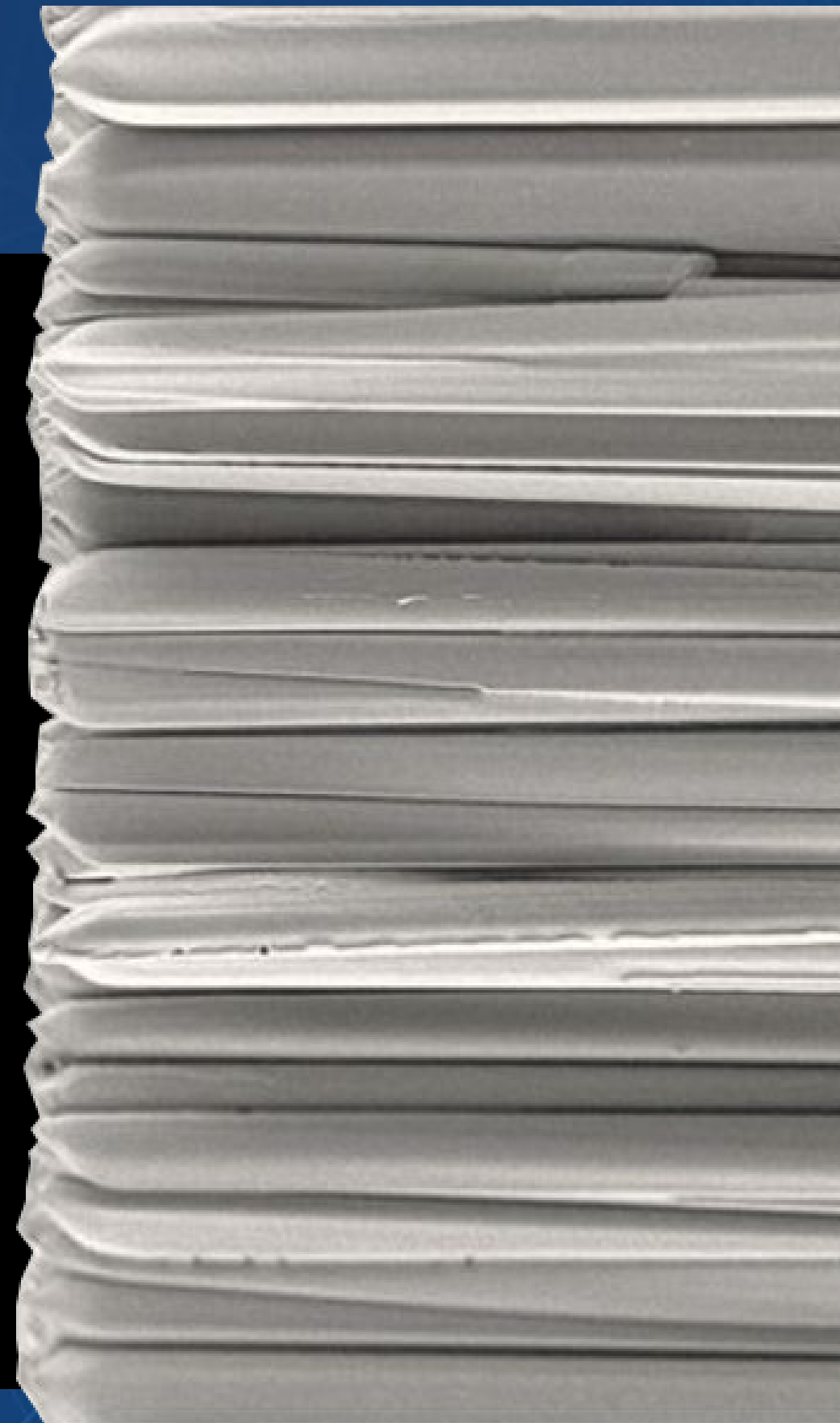
Cross-section of CsI scintillators Needle-shaped crystals
