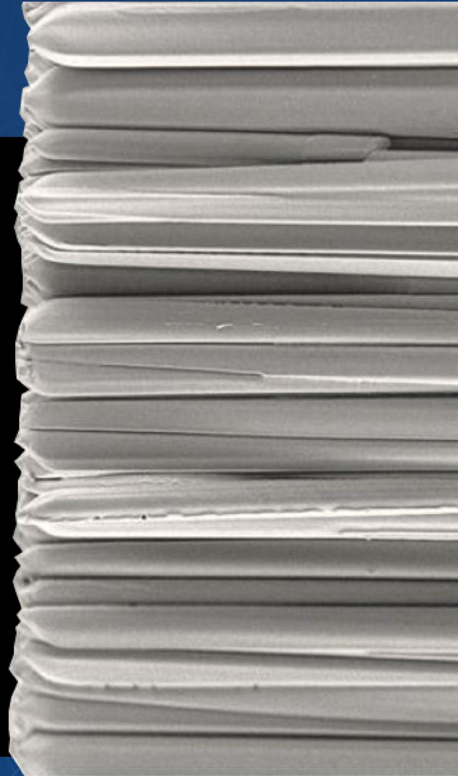
*Cross-section of CsI scintillators
